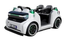
Schaeffler Paravan specializes in the development of fail-safe drive-by-wire systems. Space Drive is a key technology for automated/autonomous driving in level 4 and 5 with world-wide road approval. The system is an electronic interface that operates vehicle steering, accelerator, and braking, thus enabling autonomous driving for a wide range of applications.
